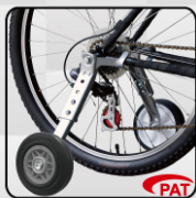
Heavy Load Training Wheels SM-902-QW Bike size: 16"- 24" bicycles. Stay size: 5m/m steel plate stay. Wheel size: 5" Rim: Bearing & Plastic Tire: Rubber tire.
