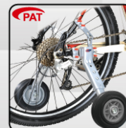
Heavy Load Training Wheels SM-902-RW Bike size: 20"- 26" bicycles. Stay size: 5m/m steel plate stay. Wheel size: 5" Rim: Bearing & Plastic Tire: Rubber tire.
