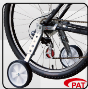
Heavy Load Training Wheels SM-901-QW Bike size: 20"- 26" bicycles. Stay size: 5m/m steel plate stay. Wheel size: 6" Rim: Bearing & Plastic Tire: Rubber tire.
