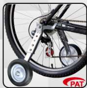
Heavy Load Training Wheels SM-903-QW Bike size: 20"- 26" bicycles. Stay size: 5m/m steel plate stay. Wheel size: 6" Rim: Bearing & Plastic Tire: Rubber tire.
